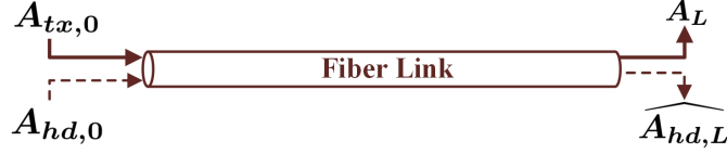
Fig. 3. Diagram of re-transmitting the HD data at the transmitter side and obtaining the received signal \widehat{A}_{hd,L} .
