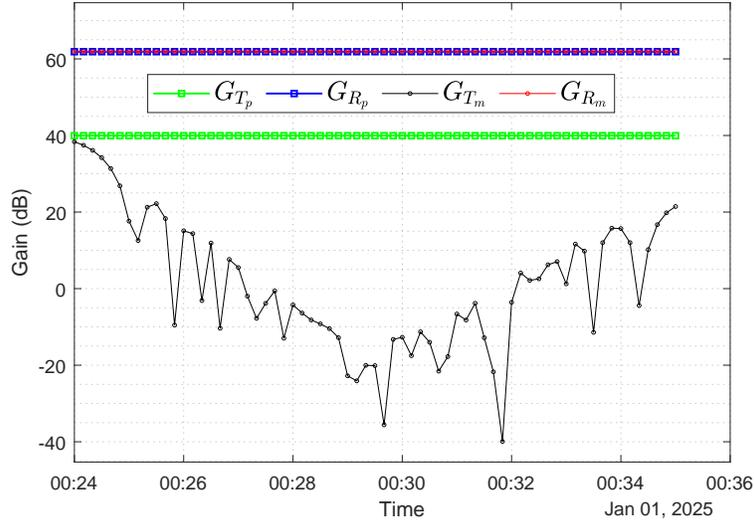
Fig. 4. Transmitting and receiving parabolic antenna gains as a function of time for the RF-based WPT realized at LSP and Malapert Mountain.
