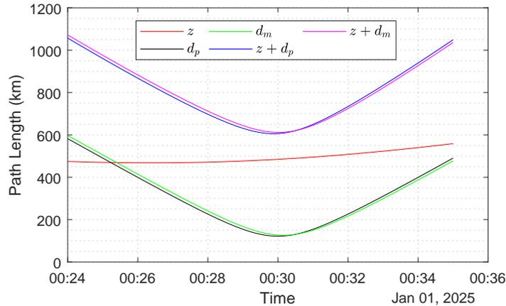
Fig. 8. Time-varying point-to-point path lengths ( $z$ ,  $d_p$ ,  $d_m$ ) and end-to-end path lengths ( $z + d_p$ ,  $z + d_m$ ) that are used for the computation of end-to-end hybrid harvested power.
