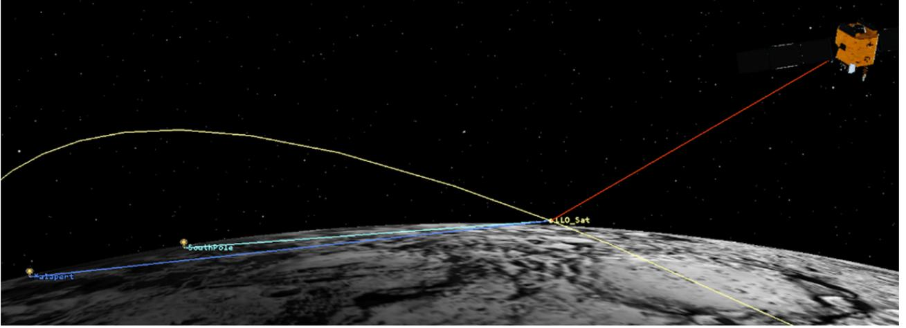
Fig. 1. In the first hop, SPS transfers laser power to the LLO satellite. This laser power is harvested by the solar array attached to the LLO satellite and is used as a relay power. In the second hop, RF-based WPT is realized between the LLO satellite and parabolic antennas located at LSP and Mons Malapert regions.
