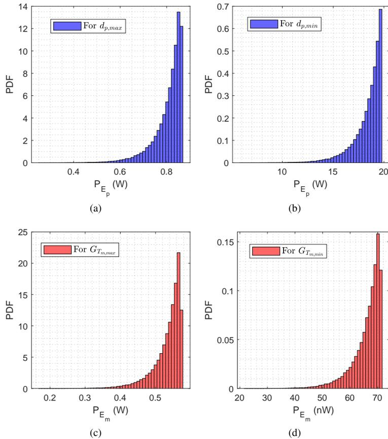
Fig. 9. Stochastic behaviours of (a) harvested power  $P_{E_p}$  for the maximum distance  $d_p$ , (b) harvested power  $P_{E_p}$  for the minimum distance  $d_p$ , (c) harvested power  $P_{E_m}$  for the maximum gain  $G_{T_m}$ , and (d) harvested power  $P_{E_m}$  for the minimum gain  $G_{T_m}$ .
