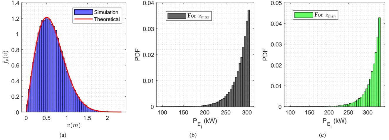
Fig. 7. Stochastic behaviours of (a) the pointing error  $v$  on the circular solar array, (b) harvested power  $P_{E_l}$  for the maximum  $z$ , and (c) harvested power  $P_{E_l}$  for the minimum  $z$ .
