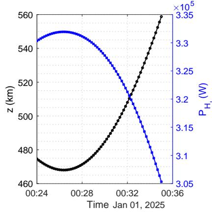
Fig. 5. The inversely proportional relationship between harvested power  $P_{H_l}$  by the LLO satellite and SPS-LLO satellite LoS distance  $z$  in FSO-based WPT.
