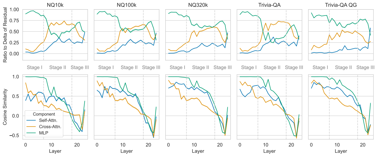
Figure 3: Proportion that each component’s output contributes to the change in the residual stream (top) and cosine similarity of each component output with the layer output (bottom), displayed per layer. The models follow a similar trend: high MLP contribution in Stage I and III, cross-attention peaks in Stage II, the cosine similarity of all components is negative in Stage III.
