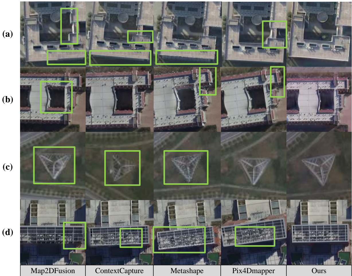
Fig. 7: Comparison between those commercial software and our method, conducted on the NPU DroneMap dataset. Our approach better represents occlusion relationships and scene details. We mark the problematic areas in the images above with green borders.
