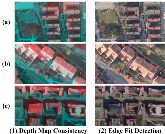
Fig. 8: Verification of the consistency between the depth map and TDOM. Column (1) replaces the R channel of the orthophoto with the depth map, and column (2) overlays the edges onto the orthophoto, which are extracted from the depth map using the Canny edge detection algorithm.
