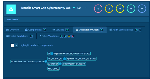
Fig. 7. Dependency graph of Tecnia’s Smart Grid Cybersecurity Laboratory.
