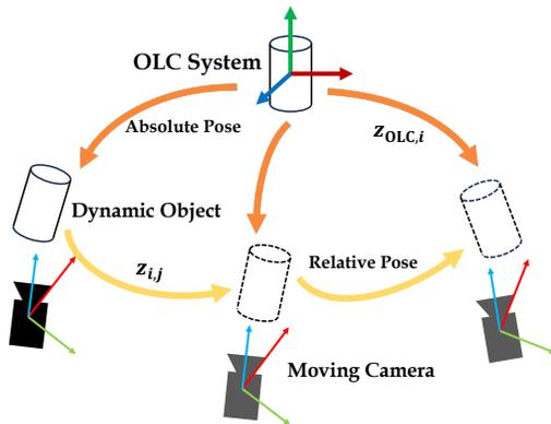
Fig. 3: Pose graph Optimization. The orange arrows represent absolute pose edges  $(OLC, i)$  and the yellow arrows represent relative pose edges  $(i, j)$ . In the OLC space, the object’s center aligns with the origin and has a semantically meaningful orientation. For example, the opening of a cup or bottle aligns with the y-axis, while the front and sides of the object are aligned with the x-axis and z-axis, respectively.
