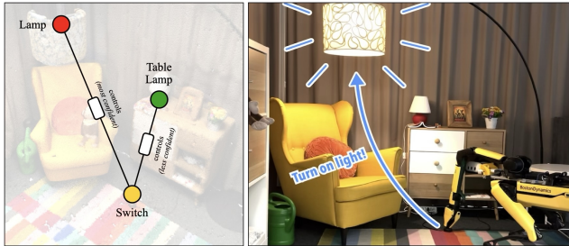
Fig. 6. Functional 3D Scene Graphs for Robotic Manipulation. Left: 3D scene and functional graph generated after querying ‘turning on the light.’ Right: Robot interacting with scene elements as guided by the functional scene graph.
