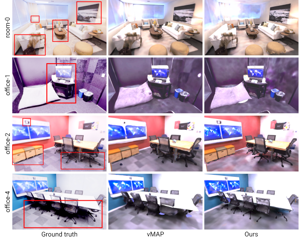
Figure 4. Examples of reconstructions with our method on different Replica scenes, compared to vMAP [35]. Our method recovers object geometry that is more faithful to the actual shapes and with better texture.
