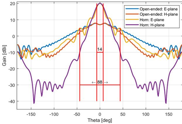
Fig. 3. Simulated radiation pattern of OWGA and horn antenna at 60 GHz
