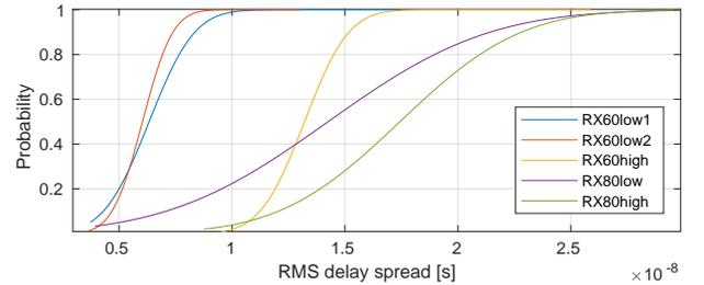
Fig. 8. Cumulative distribution function of RMS Delay Spread
