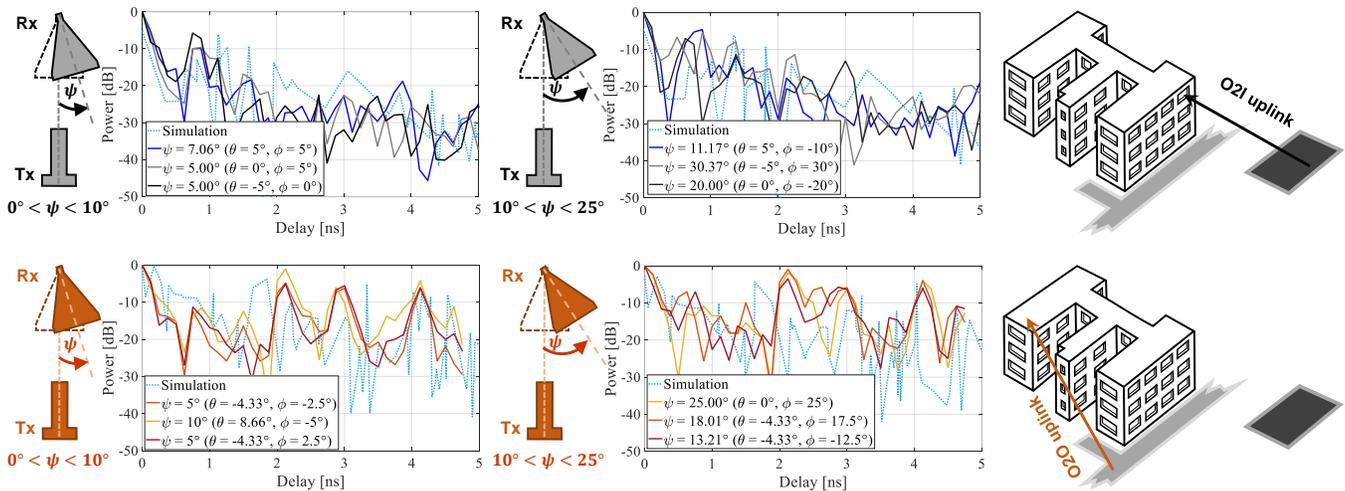
Fig. 3. Comparison of normalized PDPs for O2O/O2I uplink scenarios for two ranges of misalignment angle ( $\psi$ ). [left-top] O2I ( $0^\circ < \psi < 10^\circ$ ), [right-top] O2I ( $10^\circ < \psi < 25^\circ$ ), [left-bottom] O2O ( $0^\circ < \psi < 10^\circ$ ) and [right-bottom] O2O ( $10^\circ < \psi < 25^\circ$ ).
