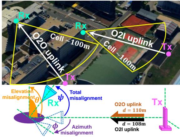
Fig. 1. Details of field measurement: [top] Aerial view of the test site showing the position of Rx in FEKT building (rooftop for O2O/ wall-mounted for O2I) and position of Tx at cell edge ( $\approx 100\text{m}$ ) at ground level, [bottom] Total Rx misalignment angle calculation from azimuth and elevation misalignment. Aerial view image courtesy: mapy.cz.
