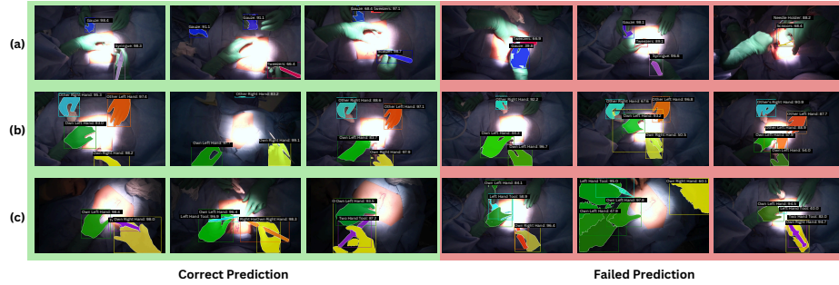
Fig. 4: Overview of the Mask2former model predictions on the three tasks. (a) Tool Segmentation task. (b) Hand Segmentation task. (c) Hand-Tool Segmentation Task.
