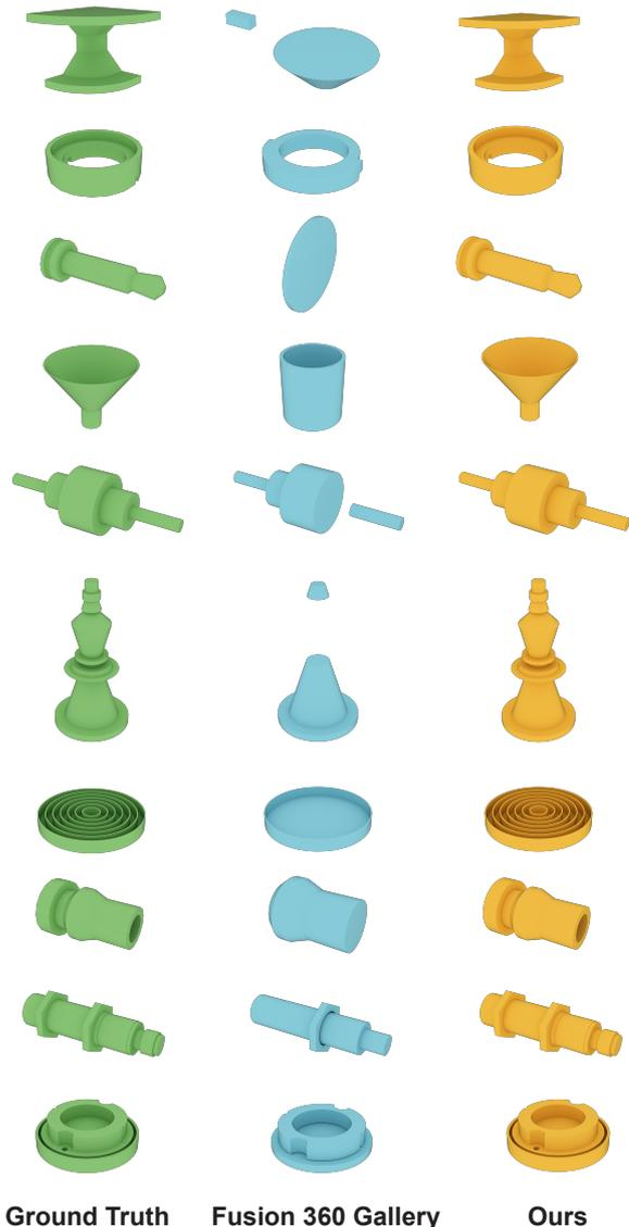
Figure 6: Qualitative comparison with Fusion 360 Gallery. Our method can generate more precise command sequence from B-Rep.
