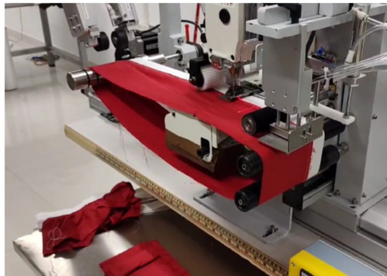
Figure 1 Outlook of Automated Stretch Elastic Waistband Sewing Machine
