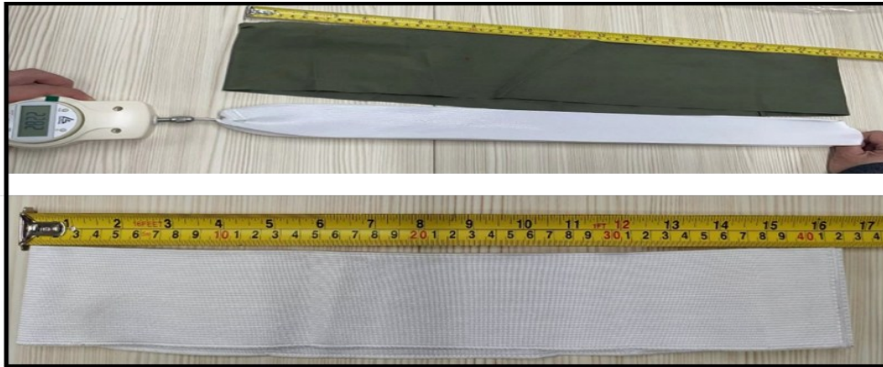
Figure 4 Elastic Band Pulling-apart Test to measure the elongation
