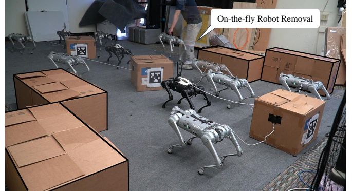
Fig. 1. Overlaid snapshots of four quadrupedal robots navigating a cable-towed load through a narrow passage using the proposed decentralized reinforcement-learning-based planner in this work. Later frames are made more transparent to highlight progression. Completing this task requires real-time coordination among teammates to adjust cable tension and avoid obstacles while navigating to the goal. The same MARL-based decentralized policy is used to flexibly control different individual robots in different team sizes. This experiment demonstrates the adaptability of the proposed decentralized policy as one robot is removed partway through the task. More experiments are shown in the video.
