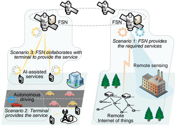
Fig. 2. Three typical scenarios of FSN-enabled edge-terminal-service integration.
