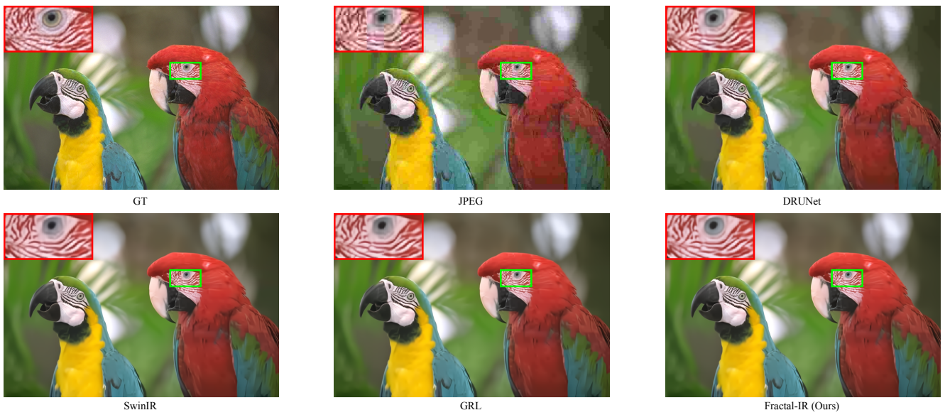
Figure G. Visual results for color image JPEG compression artifact removal on LIVE1 dataset. The quality factor of JPEG image compression is 10.
