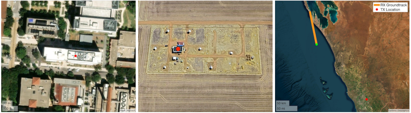
Fig. 3: Left: The spoofed location atop the former Aerospace Engineering building in Austin, Texas. Center: The actual spoofer location, a Spire Global ground station located in Perth, Australia. Right: The ground track of the Spire Global LEO satellite during the 20-second signal capture.
