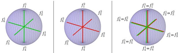
Figure 3. Geometric illustration of hyperspherical and InfoNCE losses. The hyperspherical losses (two left spheres) from (4) distributes different keypoint features  $f_j^i$  for different keypoints  $j \in [m]$  and each image  $i \in [2]$  across the hypersphere and is applied to each image separately. The InfoNCE (right side) loss from (1) aligns features  $f_j^1 \leftrightarrow f_j^2$  from matching keypoints (assuming the matching is identity here) from different images.
