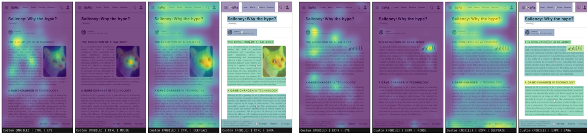
Fig. 5. Custom (MOBILE) interface heatmaps. Control group on the left, experimental group at the right. From left to right for each group: heatmaps from the eye-tracking experiment, heatmaps from the mouse-tracking experiment, saliency maps generated by DeepGaze IIE and the corresponding SaRa ranks.
