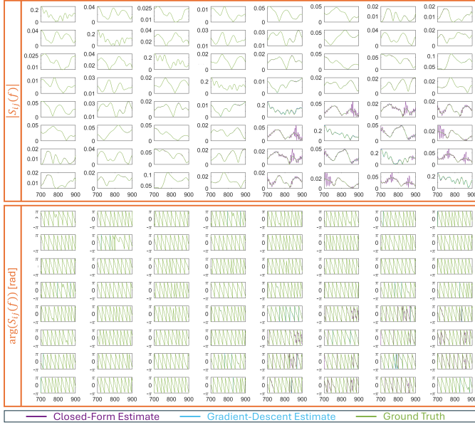
Fig. 5. Superposed display of estimated (closed form [purple] and gradient descent [cyan]) and ground-truth [green] scattering spectra for Setup 1 in terms of magnitudes [top] and phases [bottom]. The ground-truth spectra are printed on top; when only the green line is visible, the estimates are flawless.
