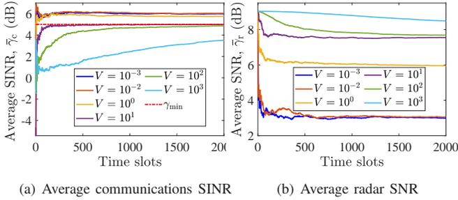
Fig. 1: Impact of the tradeoff parameter  $V$  for the *Lyapunov-SCA* method, for  $P_{\max} = 0$  dB and  $\gamma_{\min} = 5$  dB.
