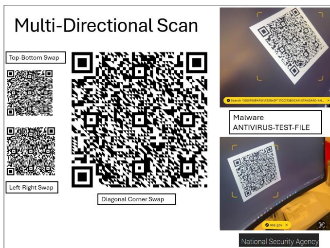
Figure 2. Single QR Codes to Support Vertical, Horizontal and Diagonal Corner Scanning with Security Test Pattern for Virus Detection (Top) and Web URL nsa.gov (Bottom)
