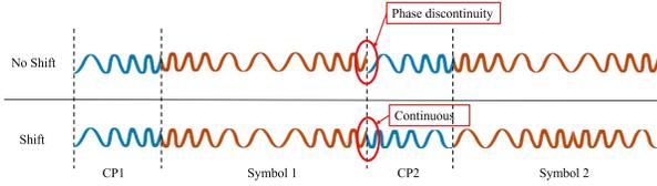
Fig. 3. CP addition before and after phase shift.
