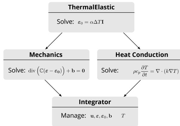
Figure 1: The MIPI schema for solving thermoelasticity.
