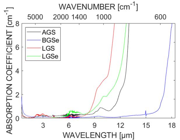
Fig. 3. Spectral dependencies of net absorption coefficients for AGS, BGSe, LGS, and LGSe.
