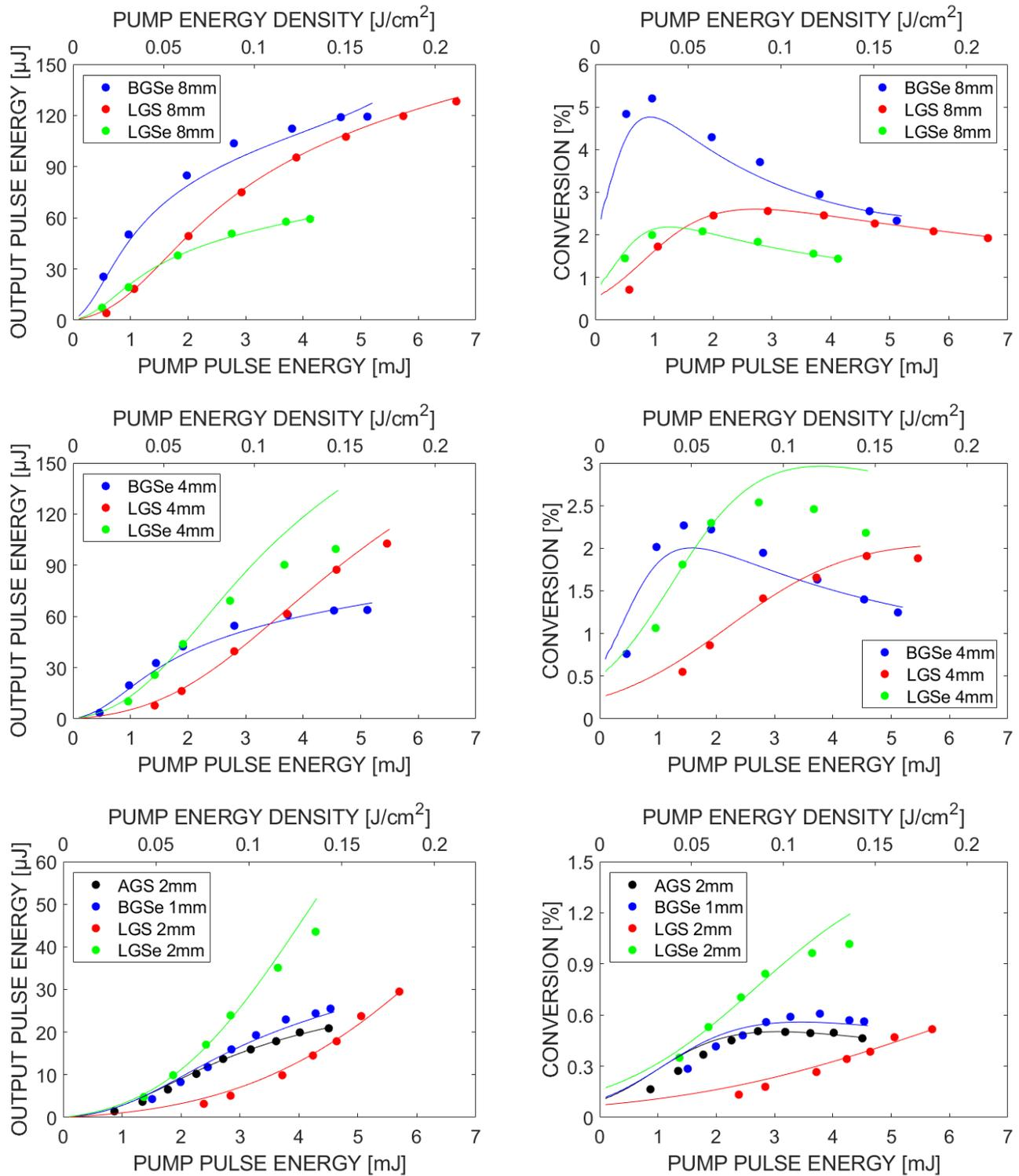
Fig. 4. Mid-IR  $\sim 7 \mu\text{m}$  output energy (left) and conversion efficiency (right) achieved with 8 mm long DFG crystals (top row), 4 mm long DFG crystals (middle row), and 1 or 2 mm long DFG crystals (bottom row). Points: measured data; line: numerical modeling.
