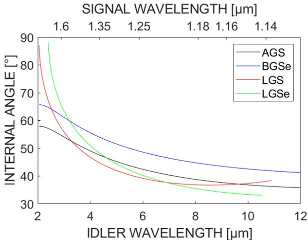
Fig. 2. Calculated phase-matching curves of AGS, BGSe, LGS, and LGSe crystals for collinear setup in principal planes according to Tab. I.
