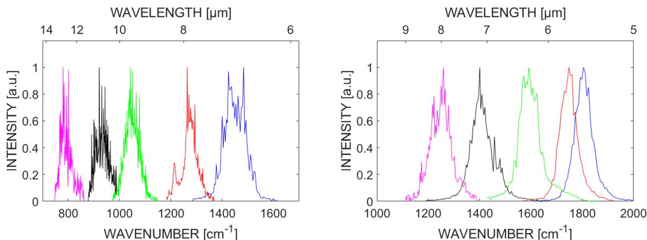
Fig. 5. DFG spectral tunability using the BGSe crystal (left) and LGS crystal (right) at high pump energy.
