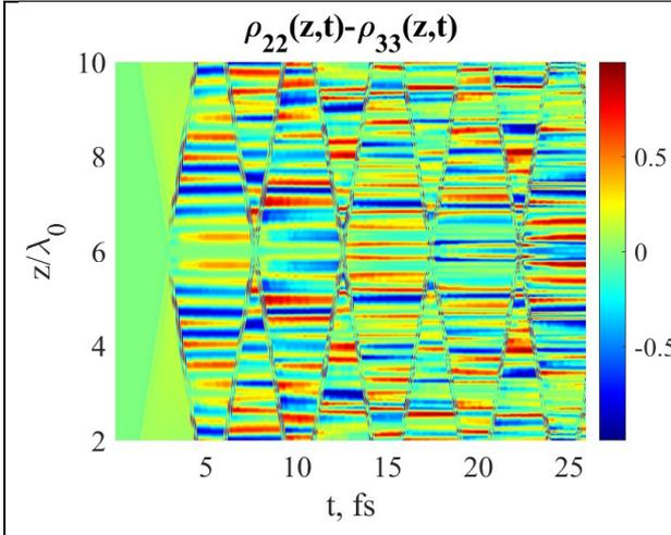
**Fig. 11.** Spatio-temporal dynamics of population differences  $\rho_{22} - \rho_{33}$  of a three-level medium.
