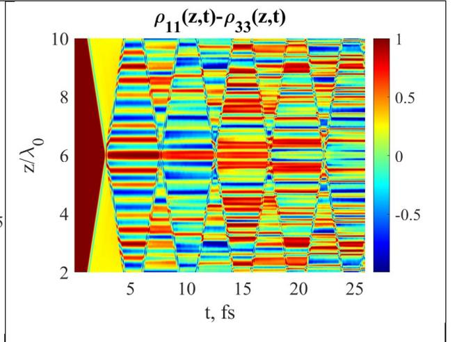
**Fig. 12.** Spatio-temporal dynamics of population differences  $\rho_{11} - \rho_{33}$  of a three-level medium.
