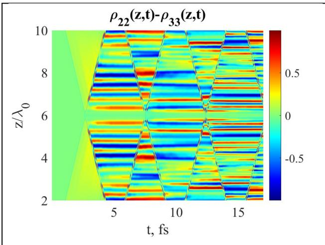
**Fig. 5.** Spatio-temporal dynamics of population differences  $\rho_{22} - \rho_{33}$  of a three-level medium.
