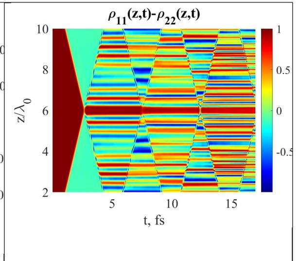
Fig.4. Spatio-temporal dynamics of population differences  $\rho_{11} - \rho_{22}$  of a three-level medium.
