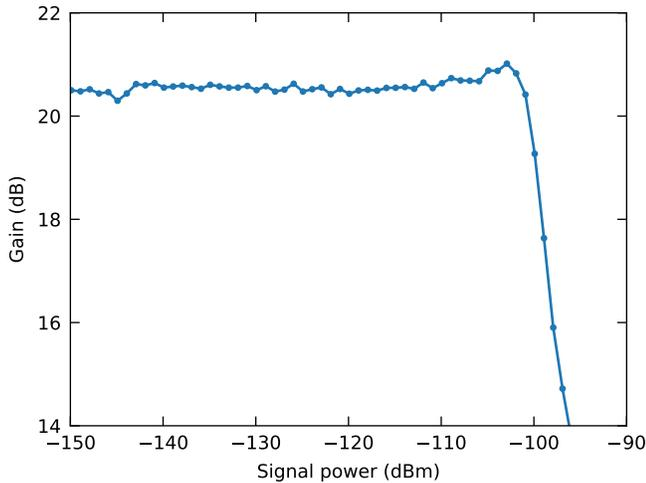
FIG. 6. Saturation power of the Tukey CP-JTWPA measured at 20.5 dB gain and 5.563 GHz. The CP-JTWPA exhibits a good gain linearity from  $-150$  dBm to  $-104$  dBm in input signal power, and saturates at  $-99$  dBm.
