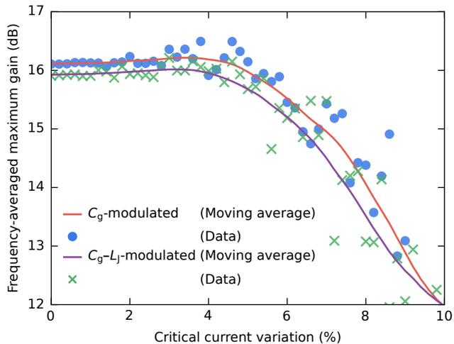
FIG. 8. Performance comparison of capacitive-only ( $C_g$ ) and capacitive-inductive ( $C_g-L_J$ ) modulated JTWPAs. The frequency-averaged maximum gain is plotted against the junction critical-current variation in standard-deviation percentage. Individual simulation points (dots) and their moving averages over twenty successive points (solid lines) show gain response over 0–10% variation, showing a similar gain degradation in both modulation schemes.
