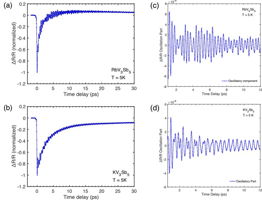
**Appendix Figure 1:** The zoomed-in plots highlighting the oscillation patterns of time-resolved reflectivity curves at 5 K for (a) RbV<sub>3</sub>Sb<sub>5</sub> and (b) KV<sub>3</sub>Sb<sub>5</sub>. (c) The oscillatory part of the measured time-resolved reflectivity curve on RbV<sub>3</sub>Sb<sub>5</sub> at 5 K in the first 12 ps. (d) The oscillatory part of the measured time-resolved reflectivity curve on KV<sub>3</sub>Sb<sub>5</sub> at 5 K in the first 12 ps.
