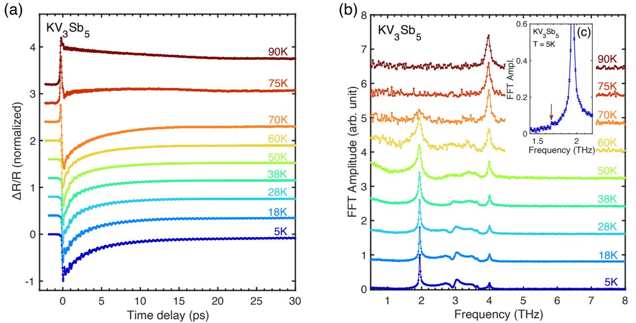
FIG. 3: **Temperature-dependent coherent phonon spectroscopy in  $\text{KV}_3\text{Sb}_5$ .** (a) Time-resolved reflectivity curves  $\Delta R/R$  at different temperatures across the CDW transition temperature. Each curve is normalized to its peak value. (b) Amplitudes of Fourier transforms of coherent phonon oscillations in (a) after subtracting the decaying background. Inset (c) shows the weak 1.68 THz mode. Curves in (a) and (b) are offset for clarity.
