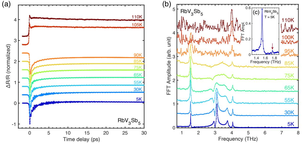
FIG. 2: **Evolution of the coherent phonon spectrum in  $\text{RbV}_3\text{Sb}_5$  vs. temperature.** (a) Time-resolved reflectivity curves  $\Delta R/R$  in the temperature range of 5 K – 110 K across the CDW transition temperature. (b) Amplitudes of Fourier transforms of coherent phonon oscillations in  $\Delta R/R$  time traces after subtracting the decay background. Inset (c) shows the weak 1.75 THz mode. Curves in (a) and (b) are offset for clarity.
