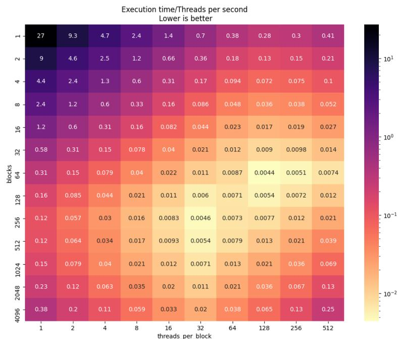
**Fig. S24 How many GPU threads for best efficiency ?** Threads/s/execution time, i.e. the previous results Fig.S23 / Fig. S22. The lower the value, the faster we get the most simulations done per second. There is a local optimum around 64-128 blocks and 128-256 threads per block, where one can obtain the most simulations done in the least amount of time spent per simulation.
