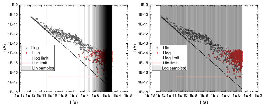
**Fig. S9 Chronoamperometry current limits depending on the type of bins.** Chronoamperometry example showing the current traces acquired linearly and logarithmically, with the associated currents limit and samples (left: linear, right logarithmic sampling). Simulation parameters: Fc free particle, 1 nm gap,  $E - E^0 = -10 \text{ mV} \rightarrow 0 \text{ mV}$ ,  $dt_{sample} = 3.3 \times 10^{-5} \text{ s}$
