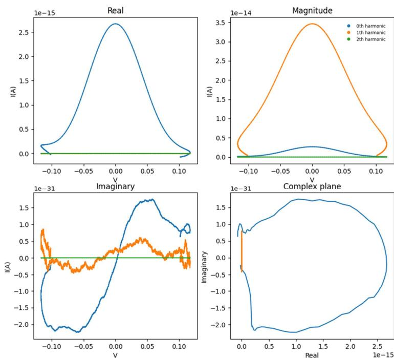
**Fig. S11 SMM experiment data treatment,** exhibiting the real and imaginary part of the harmonics of the fundamental at 2 GHz.
