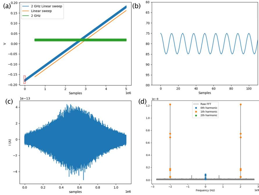
**Fig. S10 SMM experiment as implemented in QBIOL.** (a) Voltage signal applied to the electrode with its different components. (2 GHz, 5 mV, 1600 V/s)(b) Magnified voltage as marked by the red dotted rectangle in (a). (c) Resulting current over samples. (d) Fast Fourier Transform of (c). Parameters: Total time: 0.4 ms, time per sample  $\approx$  0.2 ns, output samples = 1111111, voltage samples = 5000000, Marcus-Hush rates.
