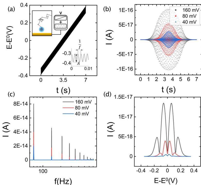
**Fig. 5 AC voltammetry QBIOL simulations** AC voltammetry with  $f = 70$  Hz,  $A = 40, 80$  or  $160$  mV,  $\nu = 0.1$  V/s,  $z_{gap} = 60$  nm. (a) Applied voltage (zoom in inset as well as schematics of the experiment). (b) Current versus time. (c) Fourier transform of the current, clearly showing well defined high harmonics for higher excitation amplitudes. (d) 4th harmonic envelope versus voltage for different excitation amplitudes.
