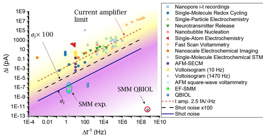
**Fig. 8 Electrochemical current limits.** Minimum faradaic current resolved  $\Delta i$  versus its measurement bandwidth  $\Delta t^{-1}$  for different electrochemical systems (adapted from [83]). See Tables S5 to S17 for numerical values and methods.
