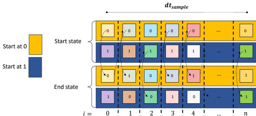
**Fig. S6 Parallel algorithm's subroutine for state history reconstruction.** With half the threads starting at 0 and the other half at 1, the actual path of the molecule is recreated by choosing one of the two threads at each step  $i$  (with  $0 \leq i \leq n$ ) spaced by  $\Delta t_{track}$ , matching the end state of a thread at  $i$  to the start state of a thread at  $i + 1$ .
