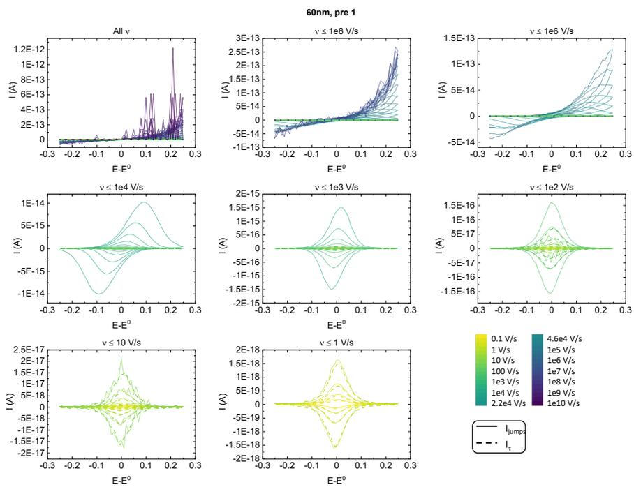
**Fig. S20 CVs in QBIOL** QBIOL-generated CV oxidation peak's voltage heatmap. Cyclic voltammograms in a 60 nm gap for Fc free particle as simulated in QBIOL, showing both current calculations methods  $I_{jumps}$  and  $I_t$  when available.
