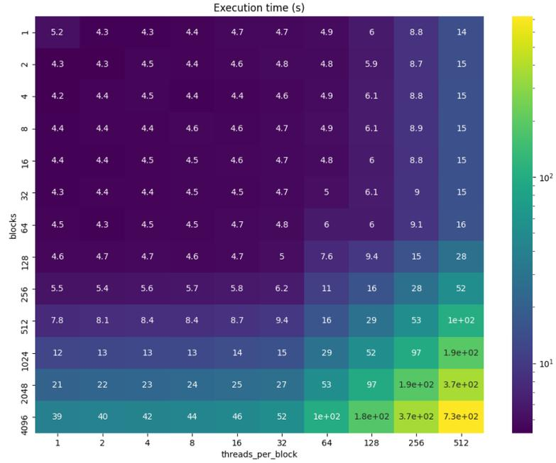
**Fig. S22** QBIOL execution time vs total number of GPU threads. Time necessary to finish the simulation (in s). The total number of threads is blocks  $\times$  threads\_per\_block.
