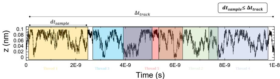
**Fig. S4 Chronological algorithm.** Example track (CV, free particle, 0.1 nm gap bounded by two walls of which one or two are electrodes) where each thread covers a different part of the track. The region covered by each thread is assigned randomly, the time window identical in duration, and depends only on the duration of the experiment (i.e. voltage step and sweep rate).
