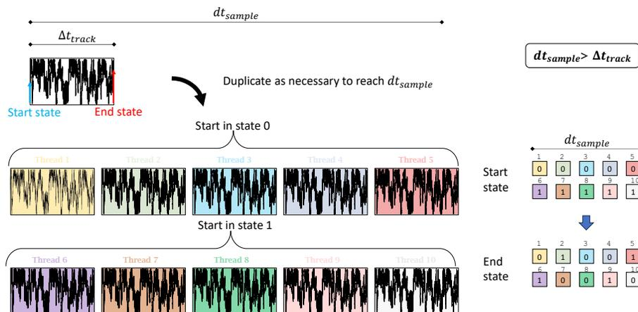
**Fig. S5 Parallel algorithm.** When the time to simulate is longer than the available MD data, the MD track is copied until it is long enough to cover the desired duration  $dt_{sample}$ . Each thread is assigned all the available MD data, and will carry on the simulation starting on 0 for half the threads and 1 for the other half. The end state of each threads is saved for further reconstruction of the state history of the molecule across the whole track.
