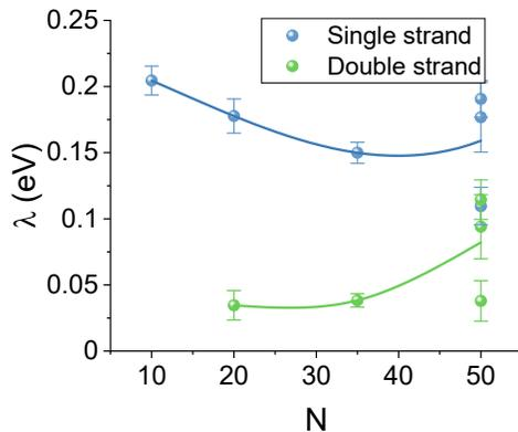
**Fig. S2** Dependency of the reorganization energy with the length of DNA. High scanrate cyclic voltammetry experiments measurements of the reorganization energy  $\lambda$  measured on ssDNA and dsDNA with different number of bases  $N$ . Lines are guides to the eye. Reproduced from [3]
