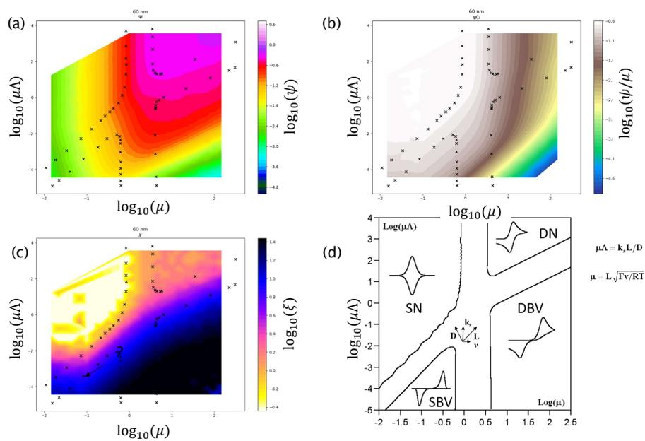
**Fig. S19 Comparison TLC model with QBIOL maps.** QBIOL-generated CV oxidation peak's current ( $\psi$ ) (a), current peak to sweep rate ratio ( $\psi/\mu$ ) (b) and voltage ( $\chi$ ) (c) heatmaps. (d) Reprint of the TLC model map (Fig. S17 for comparison).
