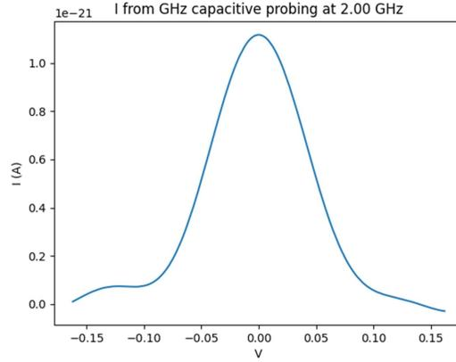
**Fig. S12 SMM output current.** Output current as obtained following the procedure described in Eq. 12 in[17]:  $I = \nu(C_{ac} - G_{ac}/\omega)/2$ .
