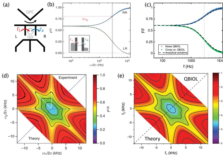
**Fig. 9 Solid-state electron counting: comparison between QBIOL and experiment.** Reproduction from QBIOL simulations of the results obtained by Ubbelohde et al. [87].
