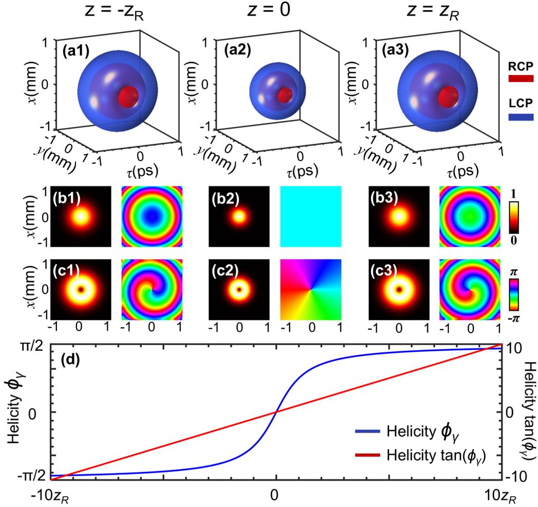
**Fig. 6** Numerical simulation of spatiotemporal skyrmion propagation in anomalous dispersive media. (a1–a3) The 3D iso-intensity (10% max) profiles of the RCP and LCP component of Spatiotemporal skyrmion at different propagation distances ( $-z_R$ , 0, and  $z_R$ ). (b1–b3) and (c1–c3) The corresponding amplitude and phase distributions of RCP and LCP component. (d) Evolution of skyrmion helicity along the propagation dimension  $z$ .
