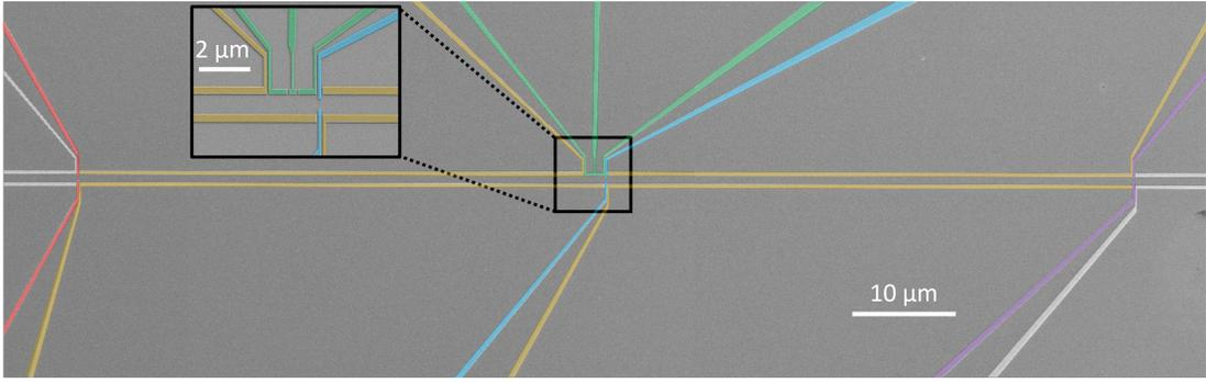
FIG. S1. **Scanning electron micrograph of the device.** False colors are used to indicate the gates used for the experiment and correspond to the ones employed in Fig. 1a. The inset is the focus around QPC2. The gates without the false colors are not used in this experiment.
