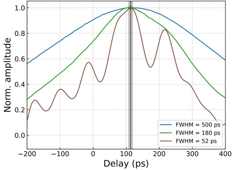
FIG. S2. **Calibration of RF line delay time using a two dimensional plasmon.** A two dimensional plasmon is excited by applying the voltage pulse with different full width at half maximum (FWHM) on the contact,  $O_i$  without applying any voltage on the gates ( $w_1$ ,  $w_2$ , QPC1, QPC2,  $g_{res}$ ). The time-resolved measurement is performed by using QPC3 as explained in the main text. The peak position does not change for different pulse lengths and is estimated to be 111(6) ps.
