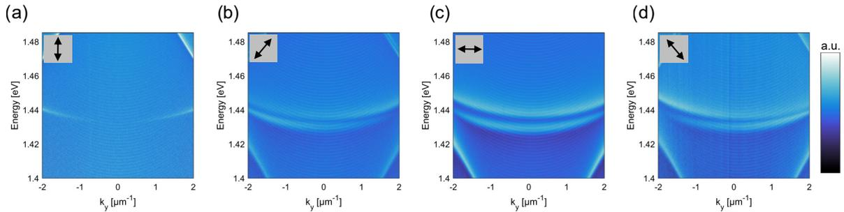
Figure S5: Polarization vorticity feature. (a)-(d) Energy-momentum dispersion measurements for any array with periodicities 475 and 350 nm along the x and y direction, respectively. The array is excited by a wide-range spectrum source for different analyzed polarization denoted by arrows. There is a clear asymmetry in the images for the two diagonal polarizations, demonstrating polarization vorticity.
