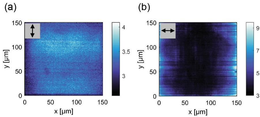
Figure S3: Real space images of lasing emission under different polarization filters for (a) TM<sub>e</sub> (vertical arrow) and (b) TE<sub>e</sub> (horizontal arrow) polarization correspond to a sample with periodicities of 480 nm and 340 nm in x and y direction, respectively. The pump fluence is 0.098 mJ/cm<sup>2</sup>.
