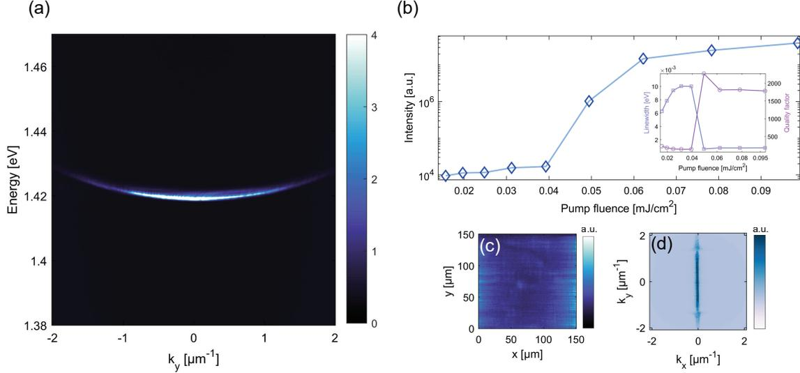
Figure 3: Lasing in the array with the  $p_x = 480$  nm and  $p_y = 340$  nm sample. The pump fluence for panel (a), (c) and (d) is  $0.078 \text{ mJ/cm}^2$ . (a) Momentum resolved lasing emission spectrum. (b) Emission power dependence on pump fluence, inset shows the full-width-half-maximum (FWHM) of the emission (squares) and quality factor (circles) with increasing pump fluence. (c) Real and (d) momentum-space of lasing emission patterns.
