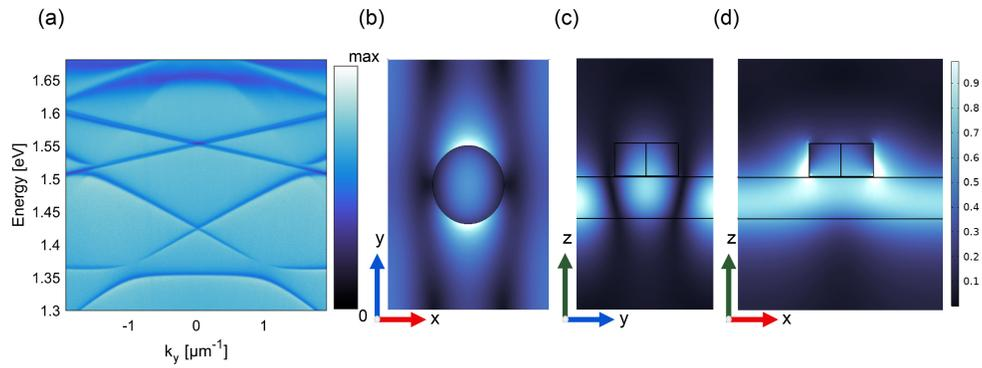
Figure S1:  $\text{TE}_w$  flat mode field distribution. (a) Transmission spectrum of an array with periodicities 340 nm in the x direction and 480 nm in the y direction.  $\text{TE}_w$  flat mode appeared at 1.35 eV. Electric field distribution of the flat mode at normal incidence ( $k_y = 0$ ), (b) in xy, (c) zy, and (d) zx plane of view. The electric field intensity is mainly within the waveguide layer and does not reach much above it (where the gain medium would be).
