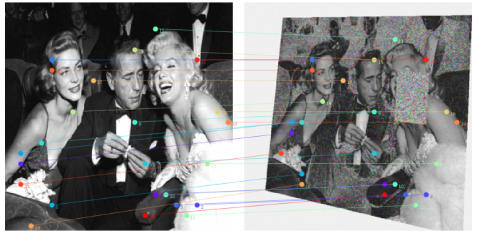
Fig. 3. ViT feature correspondences between desired image (left) and current perturbed image (right) in simulation environment.
