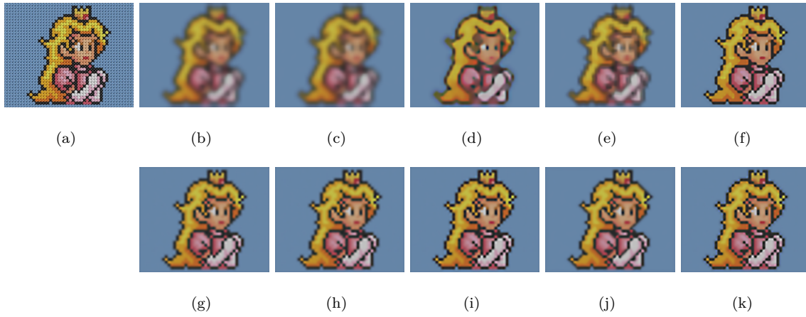
Fig. 12: Comparison of texture removal smoothing results by different filters. (a) Original image. Texture removal smoothed results: (b)-(f) GIF, WGIF, GGIF, SKWGIF, RDWGIF. (g)-(k) GH-GIF, GH-WGIF, GH-GGIF, GH-SKWGIF, GH-RDWGIF.
