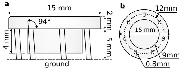
FIG. 6. **Schematic illustration of an active granular particle.** **a** Side view of the 3D-printed active granular particle, reporting heights of the particle components and the tilting angle of the legs. **b** Bottom view of the particle, showing the diameters of the cylinders forming the particles, the diameter of the legs, as well as the leg positions.
