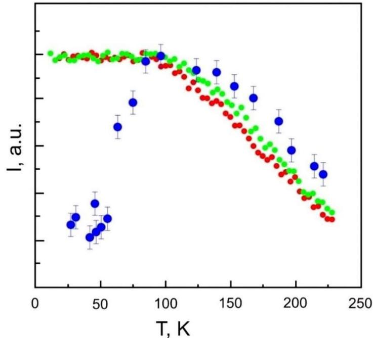
**Figure 4.** Temperature dependences of the integrated radiation intensities of  $C_{60}$  fullerite, normalized to the corresponding values at  $T = 25$  K: pure (green), intercalated  $N_2$  at 280 °C and a pressure of 30 atm (physical sorption) (red), intercalated  $N_2$  at 450 °C and a pressure of 30 atm (chemical sorption) (blue). All curves are measured in heating mode.
