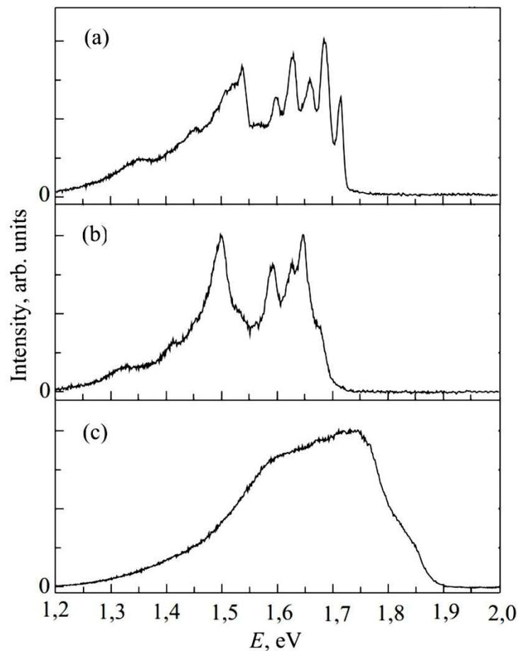
**Figure 1.** Photoluminescence spectra of C<sub>60</sub> single crystals at T=10 K, excitation with a He–Ne laser ( $E_{\text{exc}} = 1.96$  eV): pure fullerite (a); intercalated with hydrogen at 200 °C and a pressure of 30 atm (b); intercalated with hydrogen at 300 °C and a pressure of 30 atm (c). The spectra were recorded under identical conditions and were not corrected for the spectral sensitivity of the setup.
