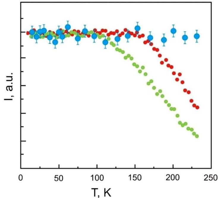
**Figure 2.** Normalized temperature dependences of the integrated radiation intensities of fullerite  $C_{60}$ : green - pure  $C_{60}$ ; red - intercalated with  $H_2$  at 200 °C 30 atm., (physical sorption); blue - intercalated with  $H_2$  at 300 °C 30 atm., (chemical sorption).
