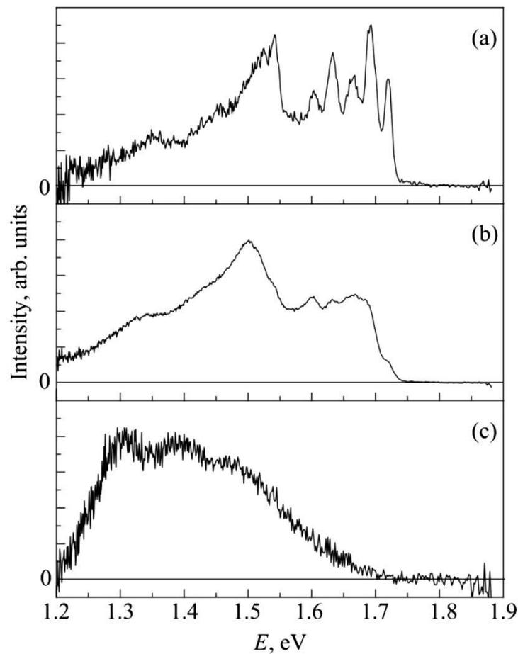
**Figure 3.** The photoluminescence spectra of a polycrystalline  $C_{60}$  samples at 30 K: (a) pure fullerite; (b)  $C_{60}$  saturated with molecular nitrogen at a temperature of 280 °C; (c) saturated with molecular nitrogen at a temperature of 450 °C. The spectra were normalized to their integral intensity and corrected for the spectral sensitivity of the setup.
