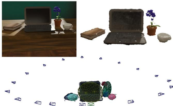
Fig. 1: DQO-MAP simultaneously reconstructs objects using Gaussian Splatting and estimates their poses with quadrics. Each object is assigned a unique ID for association and extraction.
