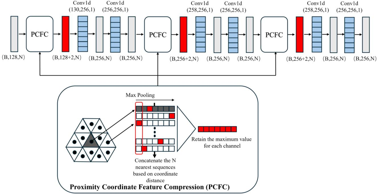
Fig. 3 Specific structure of the Feature Fusion Block.
