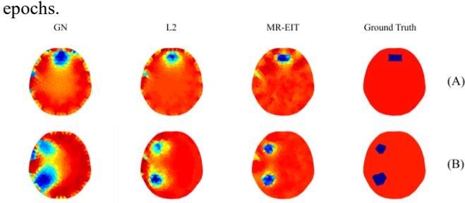
Fig. 8 The reconstruction performance of the unsupervised learning mode of MR-EIT on simulated samples.
