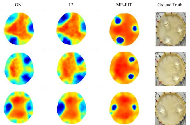
Fig. 11 The reconstruction results of the unsupervised learning mode of MR-EIT for real voltage samples on a grid with 5696 elements (high resolution).
