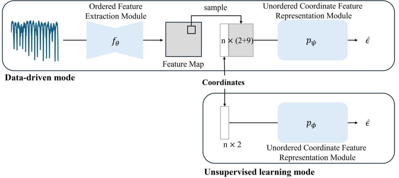
Fig. 1 The overall structure of MR-EIT
