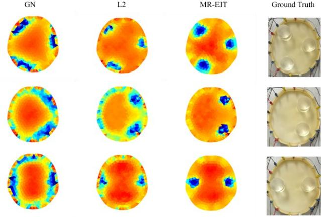
Fig. 10 The reconstruction results of the unsupervised learning mode of MR-EIT for real voltage samples on a grid with 636 elements (low resolution).
