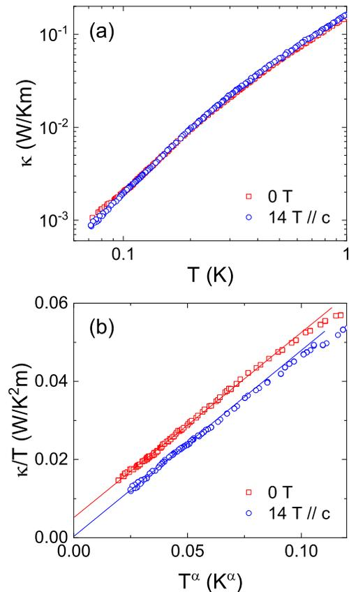
FIG. 5. (a) Low-temperature thermal conductivity of the  $\text{CeTa}_7\text{O}_{19}$  single crystal in zero field and 14 T along the  $c$  axis. (b) Ultralow-temperature data plotted with  $\kappa/T$  vs  $T^\alpha$  ( $\alpha = 1.5$  and  $1.4$  for 0 T and 14 T, respectively). The solid lines are the linear fittings to the data.
