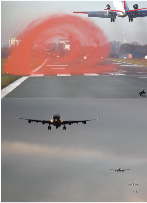
Figure 1: Top: Colored wake vortex generated by an aircraft. Bottom: Aircrafts maintaining a minimum distance during landing to avoid wake vortices.
