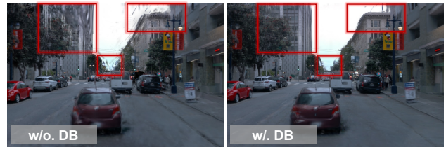
Figure 8. Effectiveness of Depth Bootstrapping. Depth Bootstrapping provides an effective gradient for the entire Gaussian field. It builds an accurate depth map enabling clearer rendering of objects. Also, it helps to reduce floaters.
