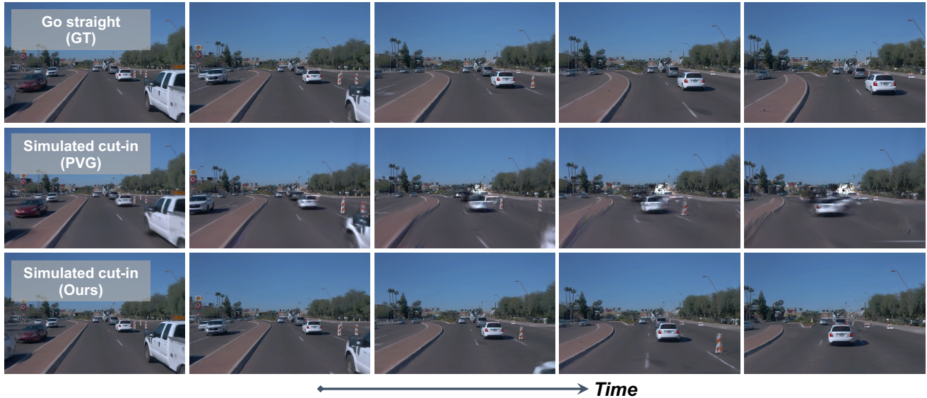
Figure 1. We simulate a cut-in case in a high-speed scenario, which is a typical functionality in driving simulators. The representative method PVG [2] fails after the lane change. We provide more video demonstrations in the attached supplementary materials.
