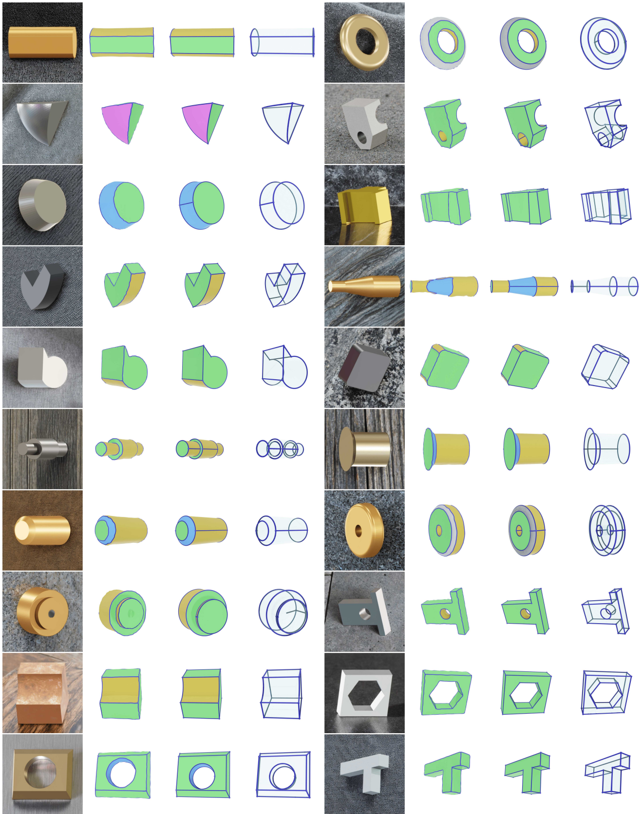
Figure 11. Reconstruction results from the given images are shown from left to right: input image, reconstructed mesh, B-reps, and their CAD vertices and edges. Different colors indicate different primitives: plane (●), cylinder (●), cone (●), sphere (●), and torus (●).
