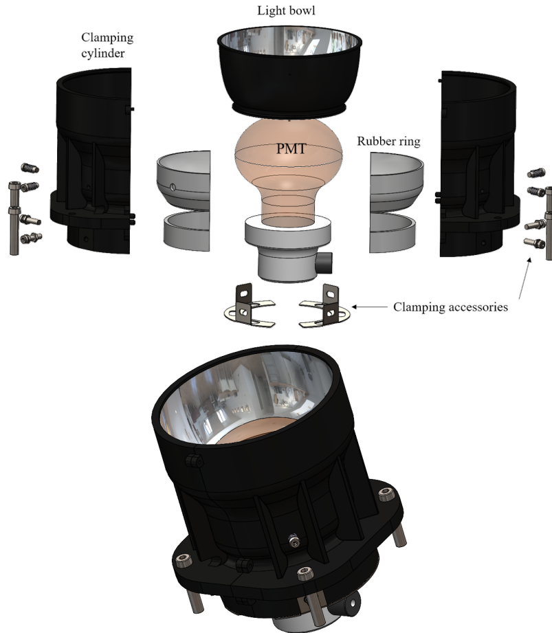
Fig 6 The disassembly and assembly diagrams of MCP-PMT and concentrator. The structure of the concentrator mainly consisting of clamping cylinder, a light bowl, silicone rubber rings and clamping accessories.
