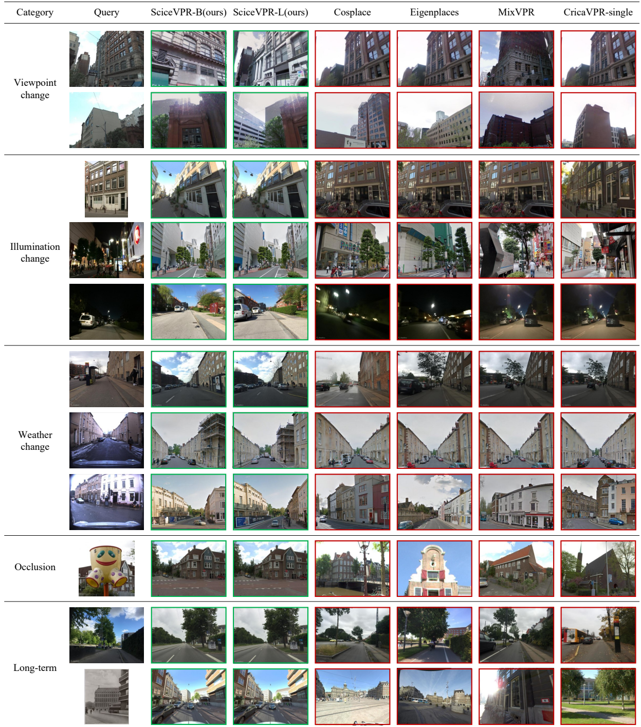
Fig. 6. Qualitative results of our SciceVPR models and the SOTA one-stage models in various challenging cases are shown. The SciceVPR models correctly recognize the true place for all the listed distinguishing queries, while the other one-stage models fail.
