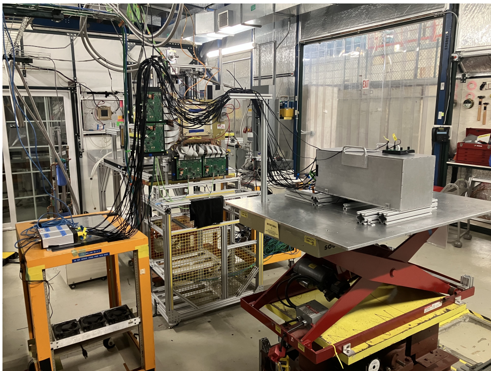
Figure 2: A photograph of the 16 channel EMCAL test module installed on the test beam motion table.
