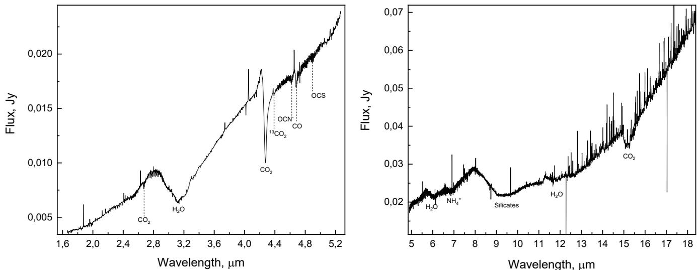
**Fig. 1.** NIRSpect (left) + MIRI (right) spectrum of the d216-0939 disk and assignments of the main spectral bands. Gas phase lines are not labelled.
