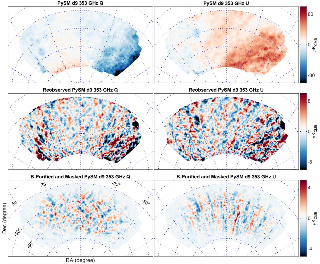
**Figure 9.** The PySM d9 maps, reobserved maps and purified & apodized maps in the BICEP/Keck sky patch at 353 GHz. Each row shows the PySM  $Q$  and  $U$  maps reprocessed by the BICEP3 beam profile, observation matrix, and purification matrix & apodization mask successively.
