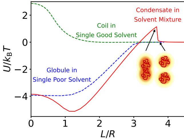
Figure 2. Potential of mean force between two polymer-cosolvent condensates in a solvent mixture, in comparison to polymers in a single good/poor solvent. The c.m. separation distance  $L$  is rescaled by the polymer radius of gyration  $R$ . The insets illustrate the two states before and after the discontinuous jump. For solvent mixture,  $\chi_{PC} = -1.7$ ,  $\phi_C^{\text{bulk}} = 0.04$ .  $\chi_{PS} = 0.0$  and  $1.0$  for single good/poor solvent, respectively.
