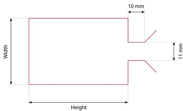
Figure S9: **Design of the inextensible pouches.** The pouches are rectangular, with an opening at one of the shorter sides. An Adobe Illustrator file, containing the red lines reported here, is used to generate the G-code. The 3D printer follows this path to seal two TPU sheets together (Methods).
