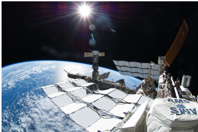
Fig. 1 The AMS-02 cosmic ray detector on board the International Space Station
